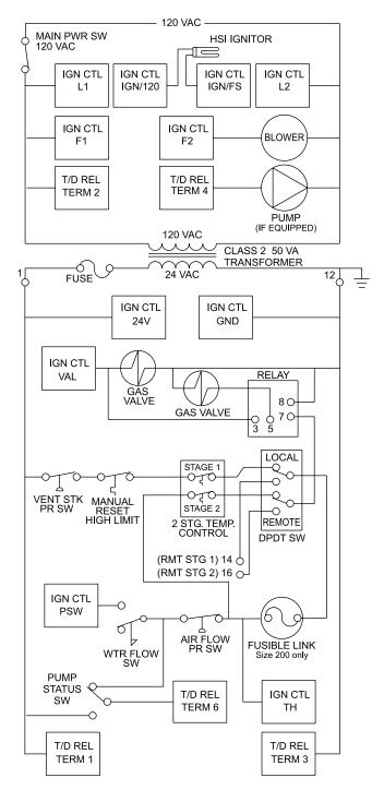
Figure 18. Logic Diagram, 2-STAGE Boiler or Water Heater.
